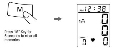
Note : The data in both memory zones (zone 1 and zone 2) will be erased if any of the batteries are removed, or if the AC adapter is disconnected from the unit or unplugged from the outlet. (It is suggested that users record their data on the Blood Pressure Log before removing or replacing batteries.)
